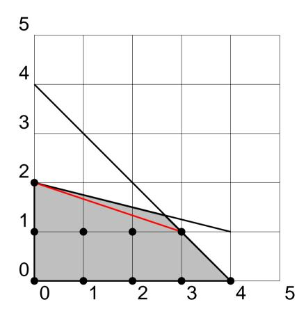
Red line is the inequality  $x_1 + 3x_2 \le 6$ . Adding this inequality gives the convex hull CH(X) of all integer solutions in X.
