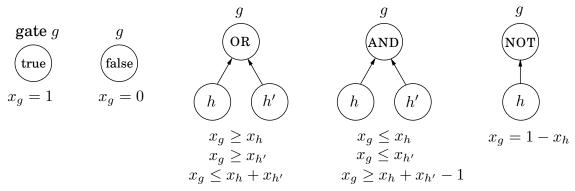
These constraints force all the gates to take on exactly the right values—0 for false, and 1 for true. We don't need to maximize or minimize anything, and we can read the answer off from the variable  $x_o$  corresponding to the output gate.
